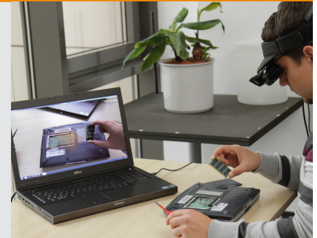
3. The display shows what the user currently sees visualized in his Head-Mounted Display
